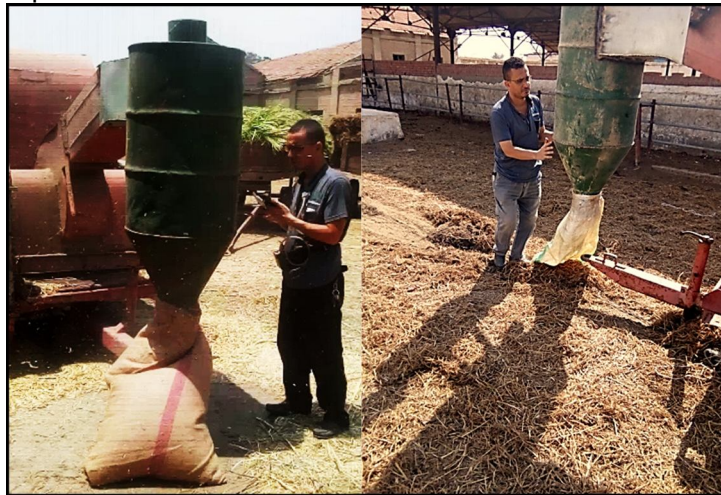
Fig. 3: Jointing cyclone inlet to thresher outlet and attaching linen sacs for collecting chopped wheat straw
