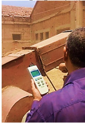
Fig.4: Measuring airstream velocity by the anemometer.
