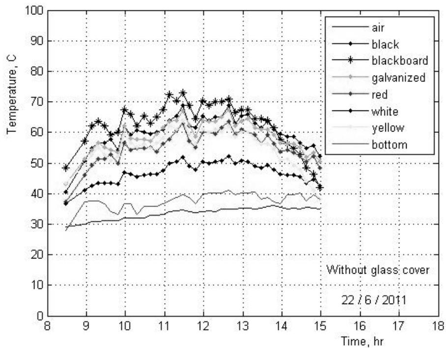
Fig.14 Temperature of different sheets with time. (Without glass cover)
