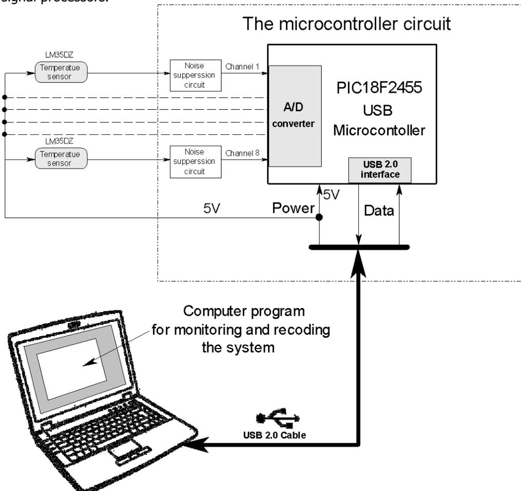
Fig. 2 A block diagram of the data acquisition system.
