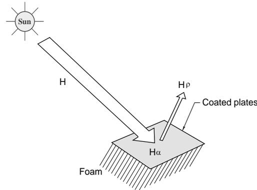
Figure 4 Solar radiation beam hitting a coated plate.
