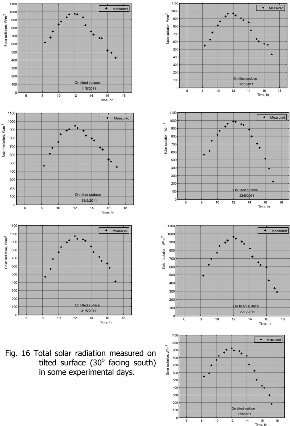
Fig. 16 Total solar radiation measured on tilted surface (30° facing south) in some experimental days.
