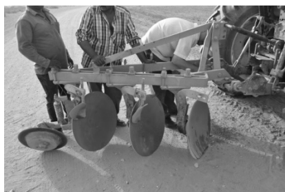
Fig. 1. Adjusting level of the used mounted disk plow.
