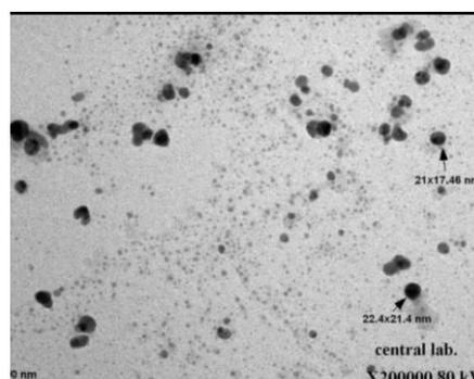
Figure 2. TEM picture of silver nanoparticles
