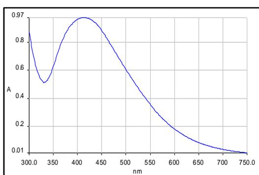
Figure 1. UV-Visible absorption spectrum of silver nanoparticles.
